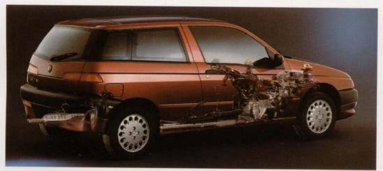
The remarkable mechanical efficiency of the Boxer engine also pays dividends in terms of long term reliability, a fact supported by the service intervals being scheduled at 12,000 miles. Both engines are fitted with three-way catalytic converters incorporating a lambda probe to neutralise exhaust emissions and naturally they run on lead-free petrol.
