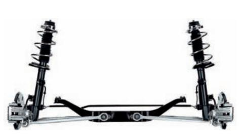
The structure of the rear McPherson suspension on the new Alfa 156 is particularly advanced both in terms of geometry and construction. The telescopic strut incorporates pressurised doubleacting shock absorbers, and the
