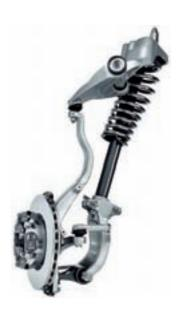
The high double wishbone suspension in the new Alfa 156 enables great lengthways wheel flexibility, without compromising roadholding while cornering and steering dynamics, guaranteeing optimum control of the tyres movements.
