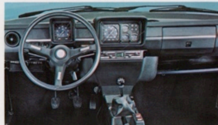
Alfetta GT instrument panel makes tachometer rightful center of attention for precision car-driver feedback. Steering wheel is adjustable for rake.
