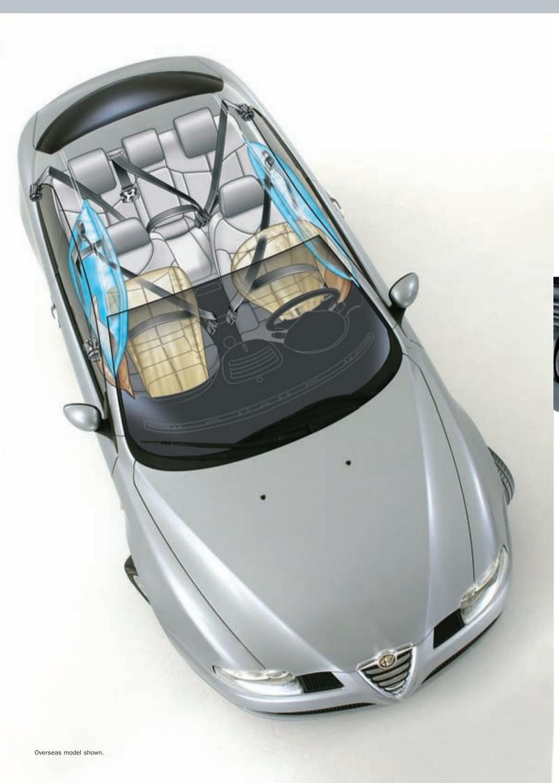
The focal element of Alfa GT's unequalled safety is the torsional rigidity of the bodyshell which helps to guarantee maximum stability and road-holding. Around its strong and progressive bodyshell, Alfa GT features an array of top class equipment: the FPS (Fire Prevention System) with tank-locking valve and inertia switch that cuts off the flow of fuel in the case of impact in some types
