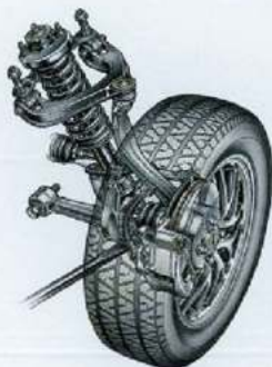
A 4-wheel, independent double wishbone suspension provides outstanding agility and responsive handling. Combined with variable, power-assisted steering, manoeuvring is practically effortless.
