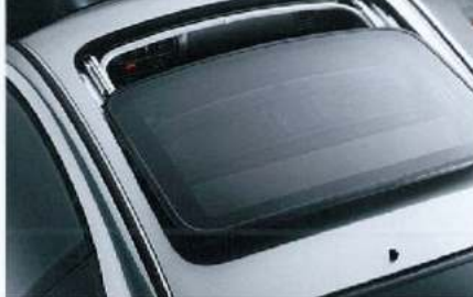
A power-operated exterior moonroof, standard on GS and GS-R models, provides more head room than interior-sliding versions.
