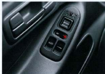
This ergonomically designed control panel, located in the driver's door, houses power controls for windows and door mirrors.
