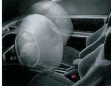
Standard dual air bags (SRS) deploy in milliseconds to help protect the driver and front passenger in frontal collisions.
