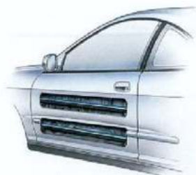
Dual side-impact steel door beams in each door give the Integra enhanced occupant protection in the event of a lateral collision.
