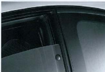
The unique pin-guide system helps reduce wind and road noise by eliminating window flex at high speeds.
